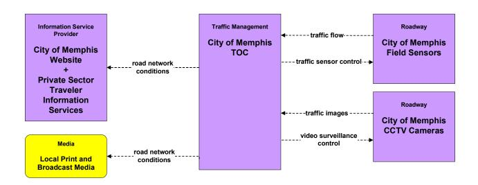
City of Memphis Field Sensors include VIVDS and any other type of vehicle detection.
